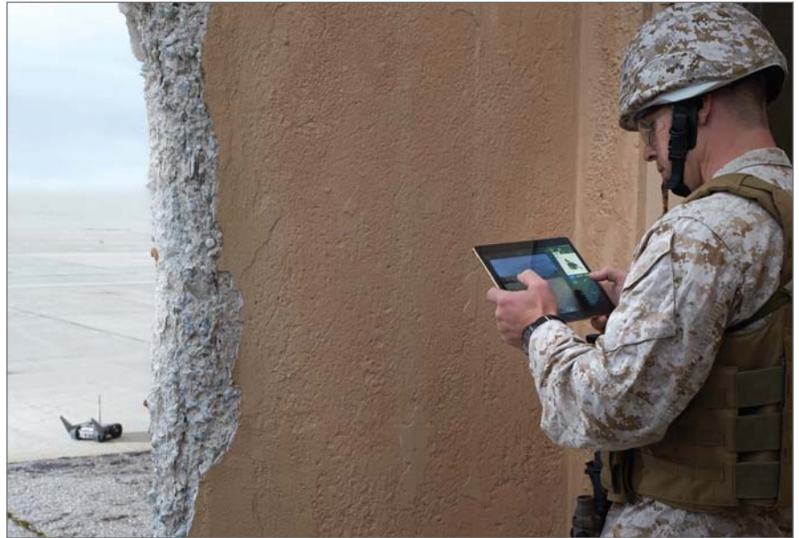
Figure 1 | The iRobot uPoint Multi-Robot Control (MRC) system uses a touchscreen tablet that runs on the Android operating system. Photo courtesy iRobot.
