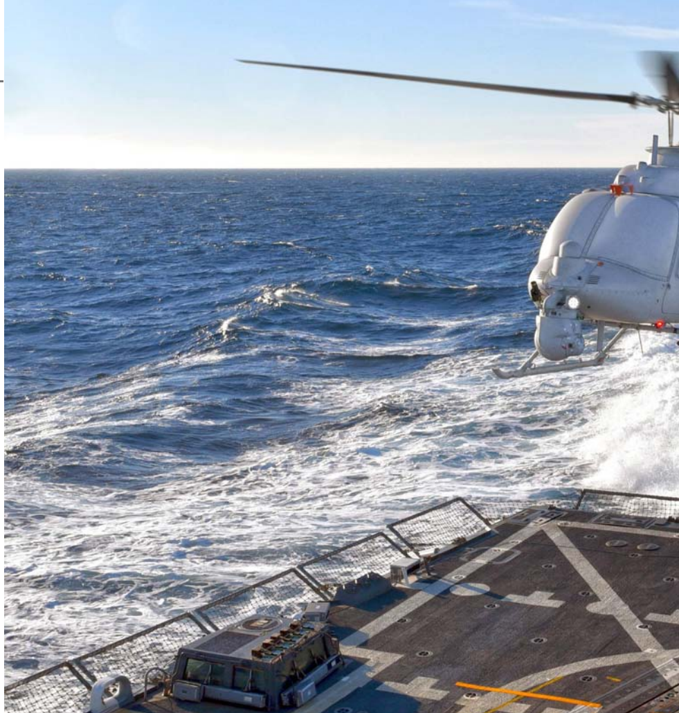
The MQ-8 Fire Scout unmanned helicopter – roughly the size of a Bell 407 helicopter and weighing 3,150 pounds – is specifically designed to operate safely from any Navy ship with a helicopter deck at sea. Photo courtesy of Northrop Grumman.
