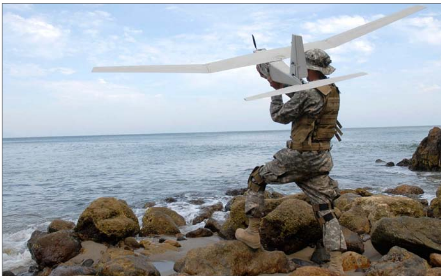
Figure 1 | The hand-thrown Puma AE has a range of 15 km. Photo courtesy of AeroVironment.
