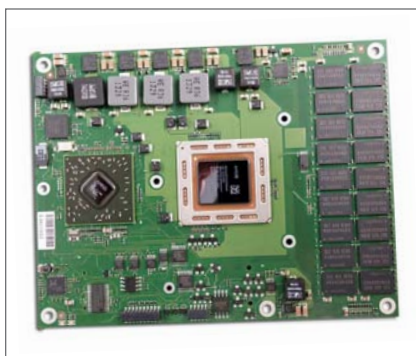
Figure 1 | The bCOM6-L1700 rugged COM Express module from GE features AMD's latest R-Series system-on-chip processor.
