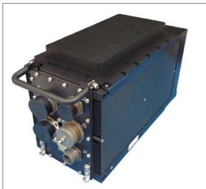
Figure 1 | The Curtiss-Wright MPMC-9351 integrated system, designed for harsh military environments, accommodates high-power 3U cards within a five-slot forced-air enclosure.
